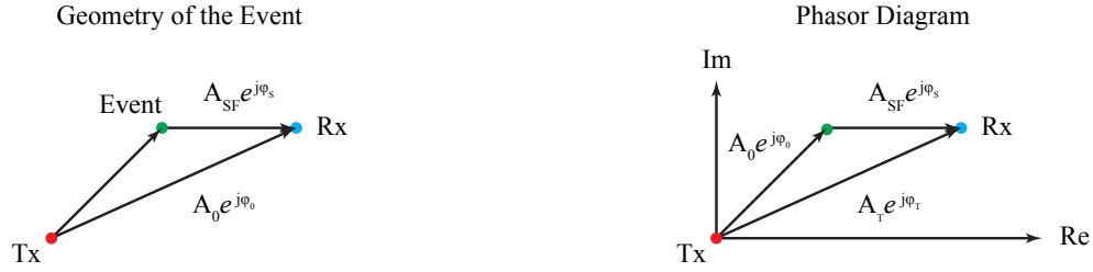
Figure 4-2. An event will create a region that scatters VLF signals. This figure shows the direct path from transmitter to receiver and an additional path from transmitter to the event and then from the event to the receiver. Each path has its own amplitude and phase.
