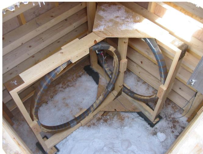
Figure 2-6. A picture of the ELF receiver at McMurdo Station, Photo by Seth White (Source:www.sethwhite.org)
